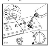
According to the finish and drying results obtained, adjust the dose of rinse aid by means of the 6 position selector (C) (position 1 - minimum dose, position 6 - maximum dose).
